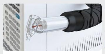
Installed at the right GC side panel. An EPC is included.
